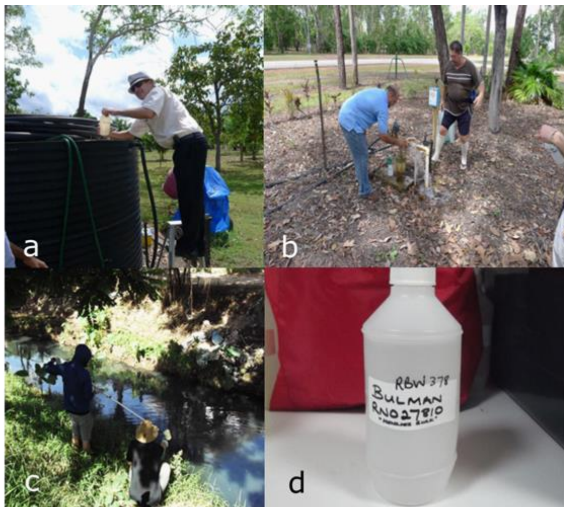
Figure 22- Water sampling for B. pseudomallei in (a) tank water (b) bore heads (c) drain water. (d) An example of an appropriately labelled water collection bottle (Images courtesy of Menzies School of Health Research, Australia).
