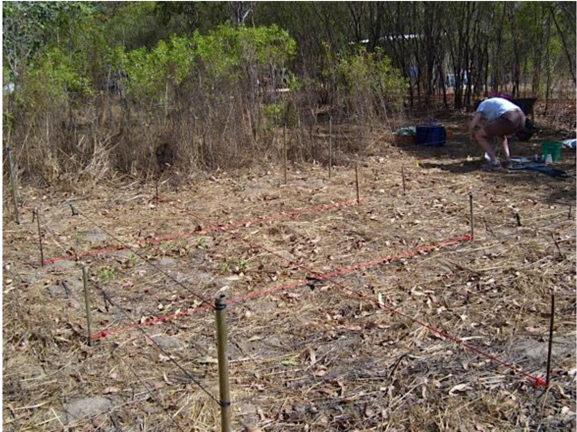
Figure 19- Example of a fixed-interval systematic grid for sampling of B. pseudomallei in soil (Image courtesy of Menzies School of Health Research, Australia).
